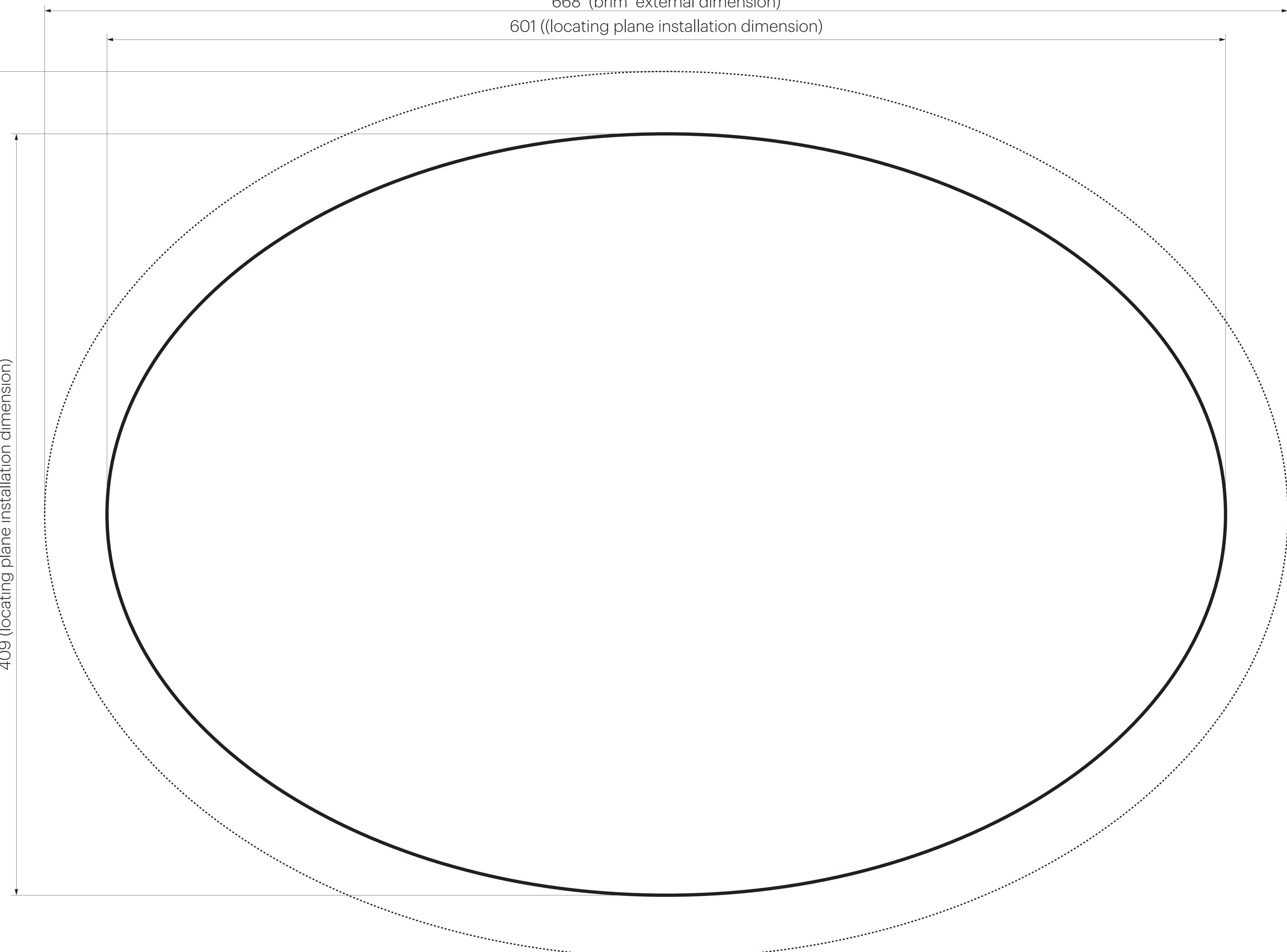
10 ~ 20 radius is recommended for chamfering for openings using stone and wood.
